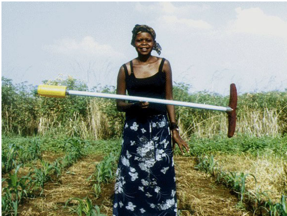
The "Weed Wipe", a really simple tool that permits late application of Roundup in a maize crop (Source: ZAMWIPE)
