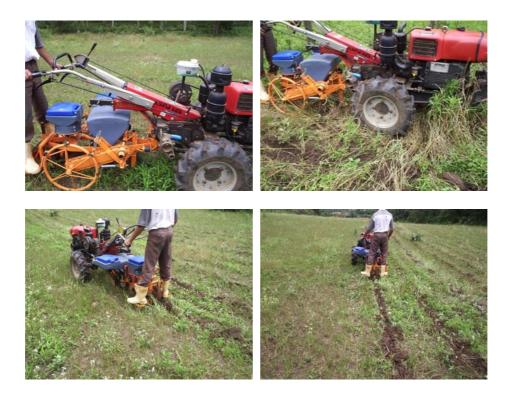
The unit has a cutting coulter disc followed by a tine opener as the soil engaging tools. A pair of inclined vee press wheels is at the back. A horizontal flat plate seed meter distributes seed. Various hitches are available for different types of 2WT.
