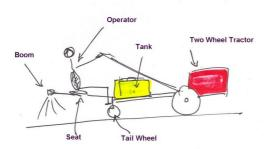
However to fabricate a unit such as in this sketch would require a custom made spray tank, which would comfortably fit under the handlebars of the 2WT
