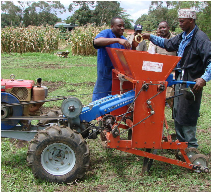
A two-wheel tractor fitted with an Australian-designed conservation agriculture planter. Photo credit CIMMYT
