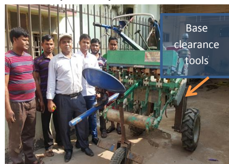
Base-clearance tools (50 cm) attached with 2WT and VMP
