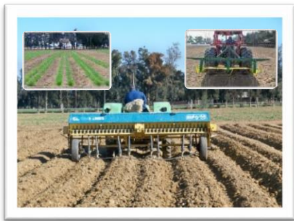
Fig: an implement was built to create beds and an old conventional seeder was used with low disturbance points, modified wheel placement and row spacing to fit the beds
