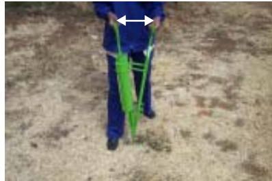
6a Spread handles to feed the seed
