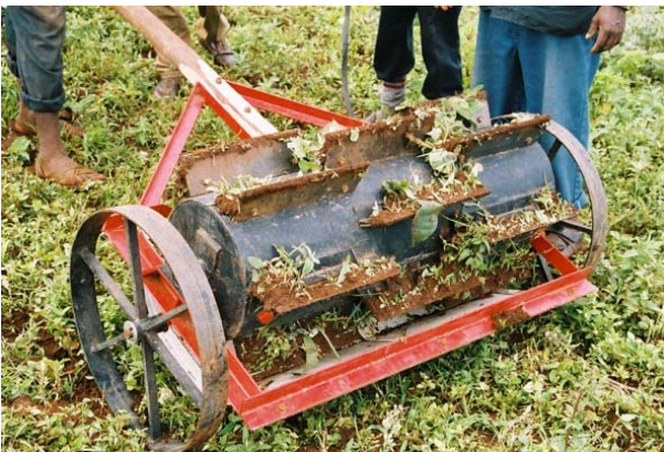
30 An animal-drawn knife-roller, turned upside-down so it can be transported Brian Sims
