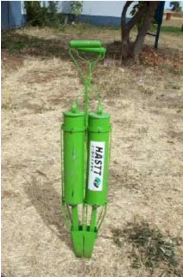
4 A jab-planter with two containers: for seed and for fertilizer HASTT, Zimbabwe
