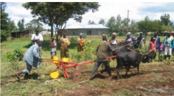
11 Testing a Fitarelli No. 12 direct planter and fertilizer distributor Josef Kienzle
