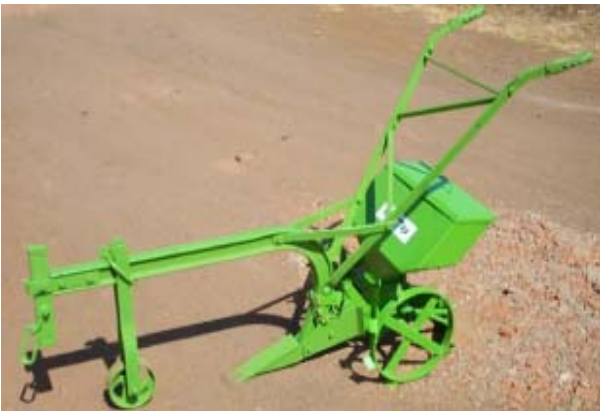
7 Simple ripper-planter pulled by two donkeys. Design by Triple W Engineering. Barney Muckle
