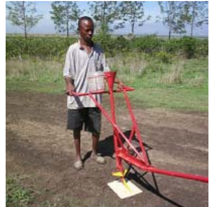
8 Oxen-pulled ripper-planter. Design by Triple W Engineering/ KARI. Barney Muckle
